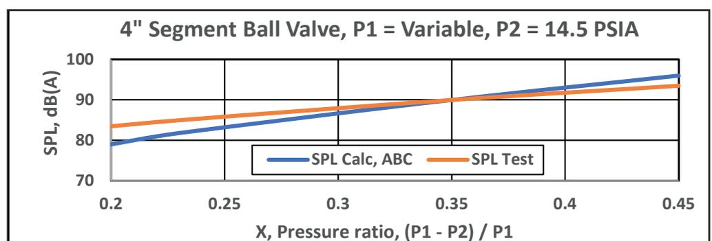
Figure 1. Comparison with an actual blowdown noise test.
